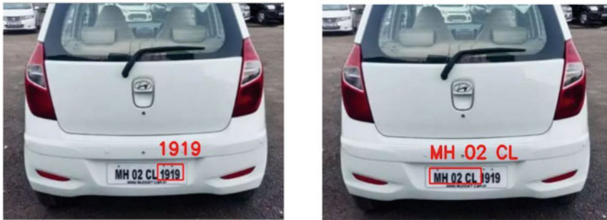
Fig. 10 License plate recognition when input is a colored image
