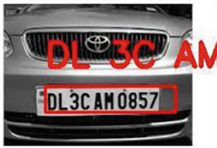
Fig. 9 License plate recognition when input is a grayscale image
