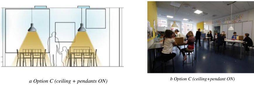
Fig. 5 Option C - Ceiling and pendant lighting activated. a Sketch depicting artificial lighting Option C. b Photo of the classroom with artificial lighting Option C activated. Image credits: Henning Larsen, Imke Wies van Mil. Photo credits: Henning Larsen, Halfdan Trolle
