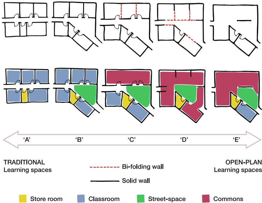
Fig. 1 Typology of spatial design (source Imms, Cleveland & Fisher, 2016. Reprinted with permission from the ILETC project)
