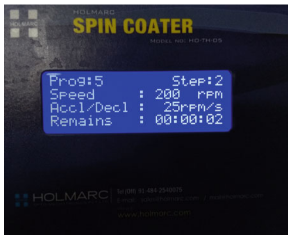
Fig. 2 Parameters setup for spin coater (fabrication of nanocomposites)
