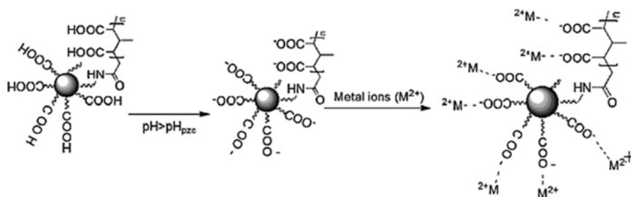
Fig. 13.6 Schematic diagram of conversion of carboxyl into carboxylate and adsorption of metallic ions by nano- \text{Fe}_3\text{O}_4 (Adapted from Gangadhar et al. 2012)
