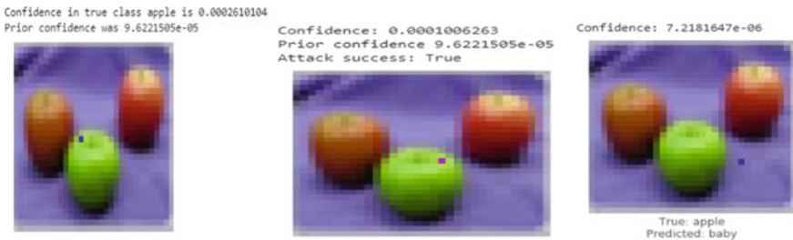
Fig. 5 Shows confidence of the model changes after adding small perturbation into the image. The middle image shows the success of attack on a single image for non-targeted attack prior confidence 9.6221505e-05 & the attack successful
