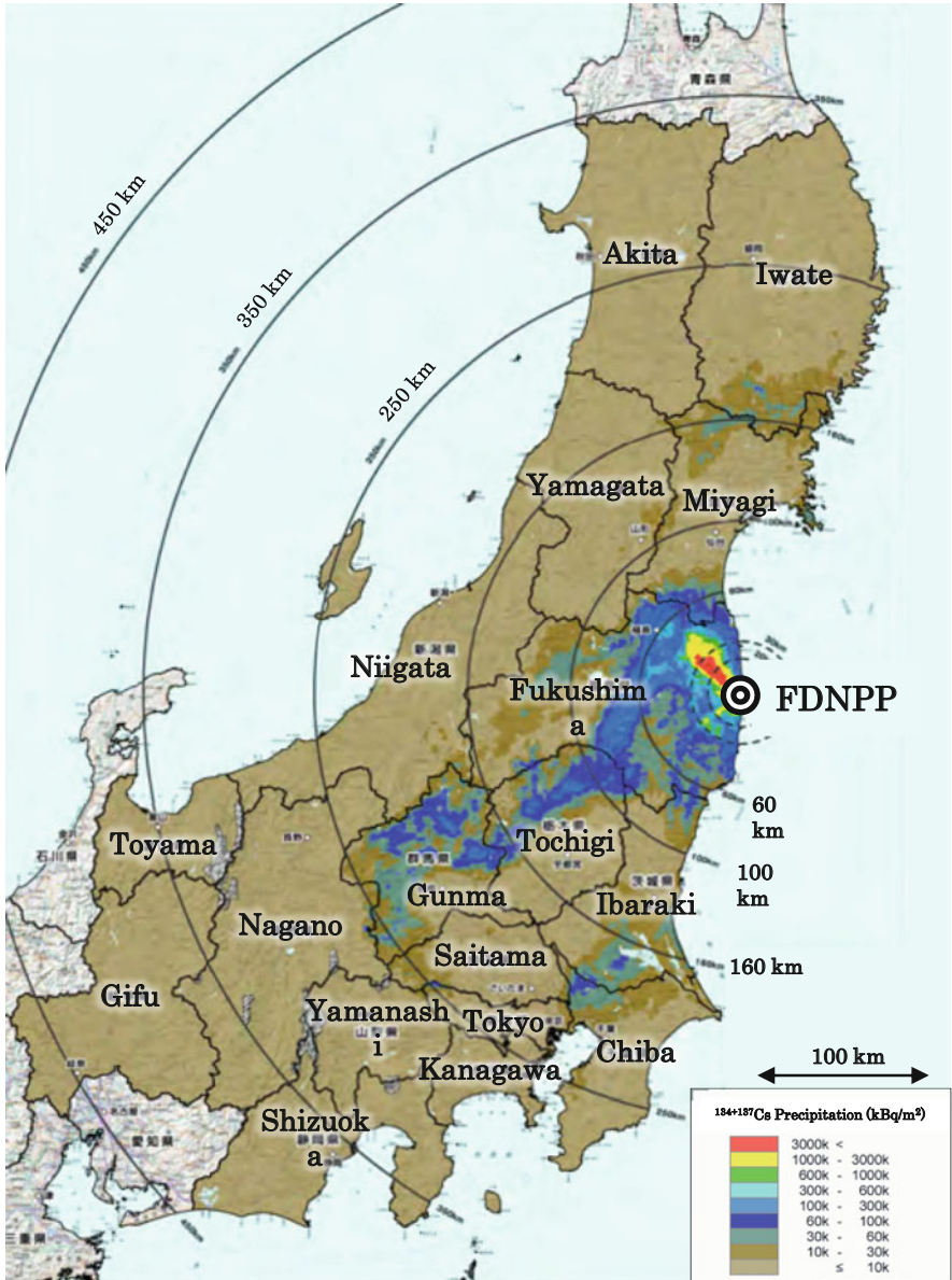
Fig. 3.2 Geographic distribution of the ^{134+137}\text{Cs} precipitation in eastern Japan. This monitoring survey was carried out by the MEXT from April to October 2011, and the results were published in November 2011 ([14] a)
