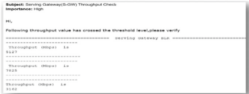
Fig. 17 Monitoring the throughput value of serving gateway (S-GW) of the 4G network in Bangalore location
