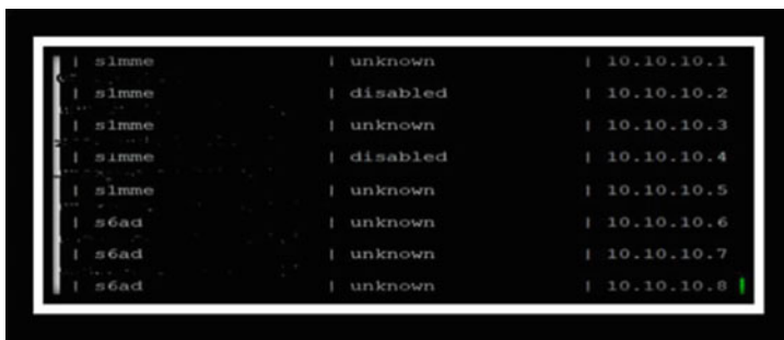
Fig. 4 Monitoring s1-mme, s6a interface in the putty server
