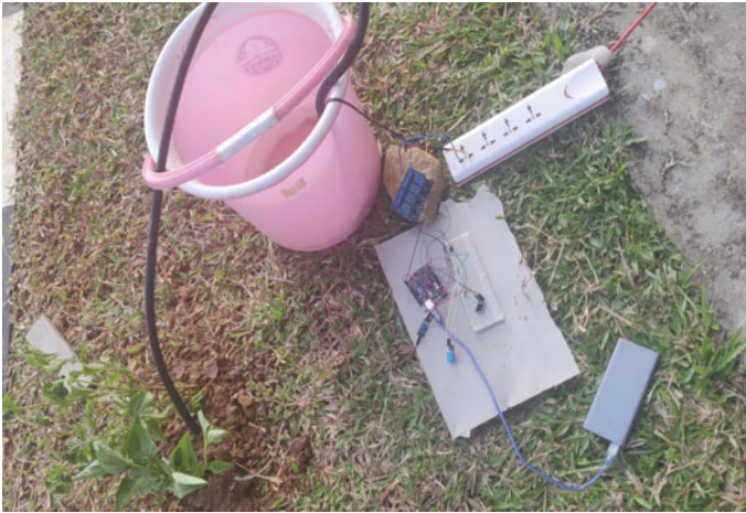
Fig. 3 Hardware implementation of smart crop monitoring and irrigation automation
