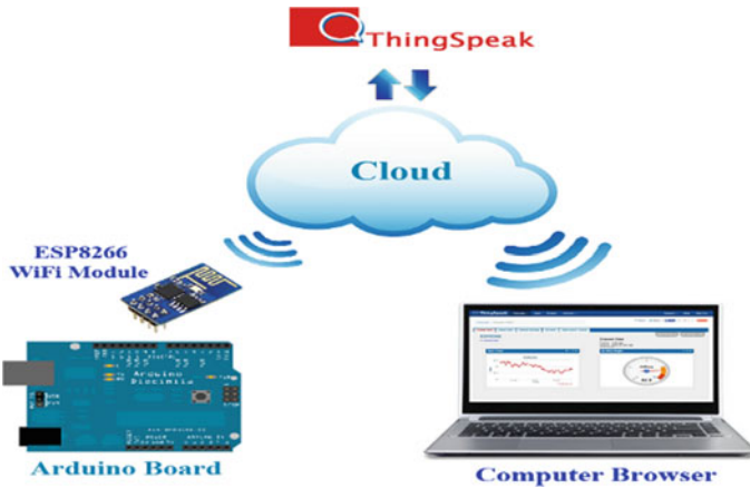
Fig. 3 Communication of Arduino with ThingSpeak
