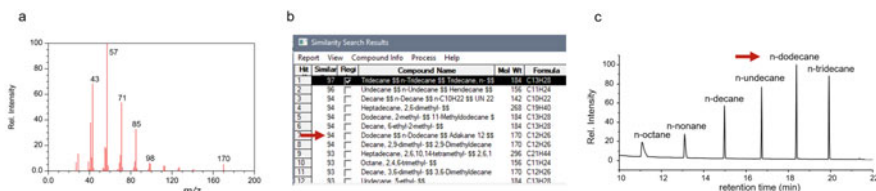
Fig. 12.4 Identification of n -dodecane. Mass spectrum of n -dodecane (a) revealed that dodecane was only at the seventh position in similarity search using NIST Library with 94% similarity (b). In order to distinguish between the single alkanes, e.g., the first hit tridecane with 97% similarity, co-elution experiments with authentic standards confirmed the identification of n -dodecane (c)
