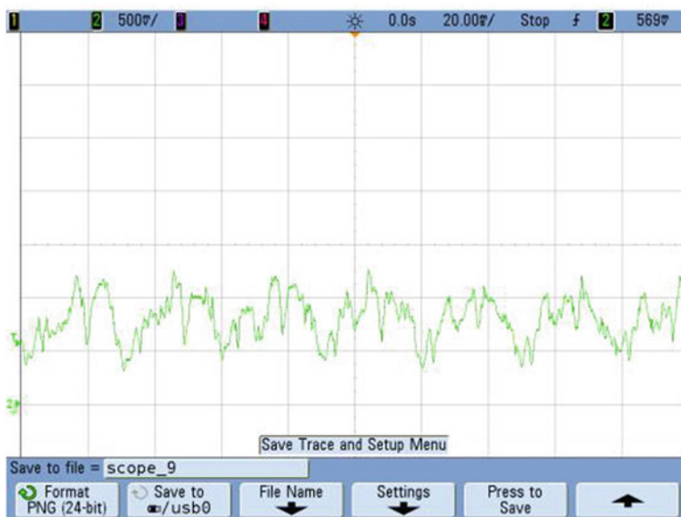
Fig. 14 Torque using ILC-SVPWM at 2000 rpm
