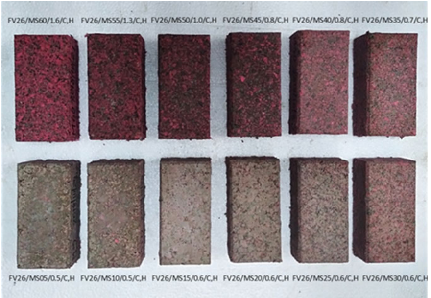
Fig. 6 Surface appearance of paving blocks
