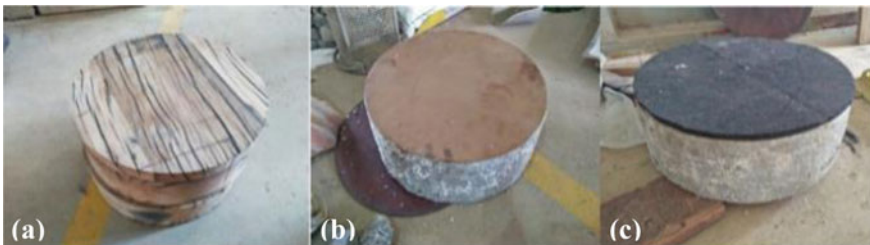
Fig. 2 Sleeper sample a Timber; b concrete; c USP
