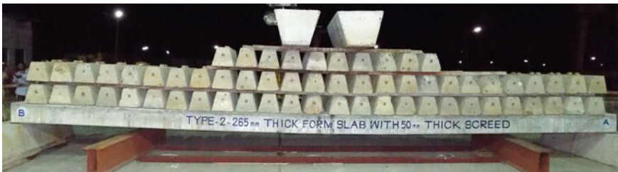
Fig. 10 The deformed shape of the specimen with screed concrete
