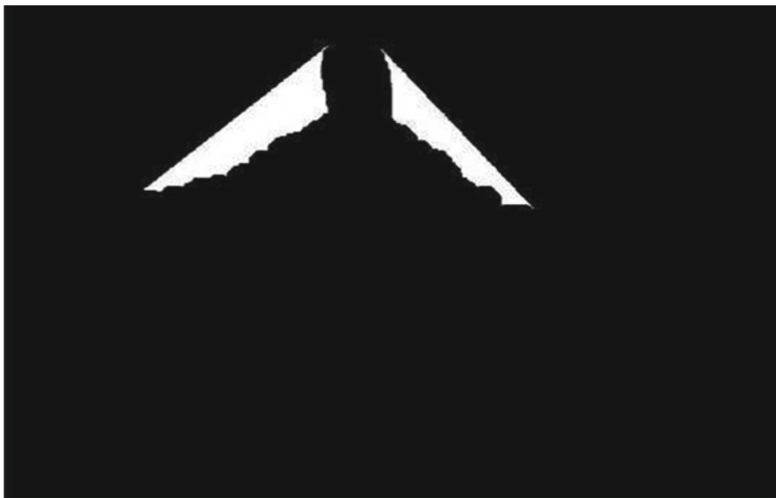
Fig. 7 Largest connected domain A_1 and A_2 in the set after the logical operation
