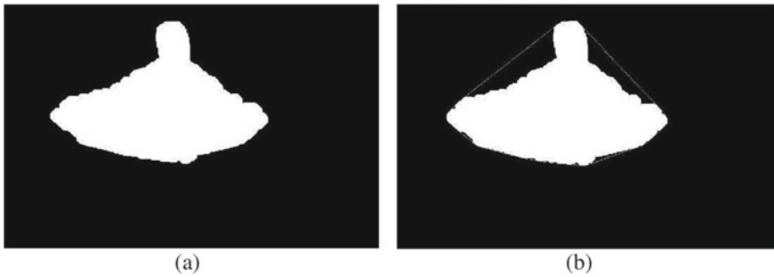
Fig. 6 Morphological processing for feature extraction: a morphology edge smooth in arc region; b convex hull detection
