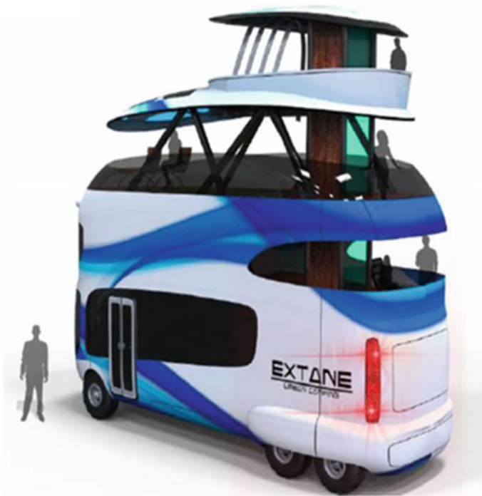
Fig. 10.4 Vertically expandable RV prototype. Source Caldicott (2017)
