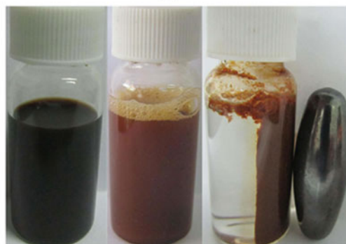
Fig. 4 a Schematic description for the preparation of magnetic nanohydrogels; b digital images of starch-maleate-magnetic nanoparticles stable ferrofluid, magnetic nanohydrogels dispersion and magnetic response of nanohydrogels (left to right)
