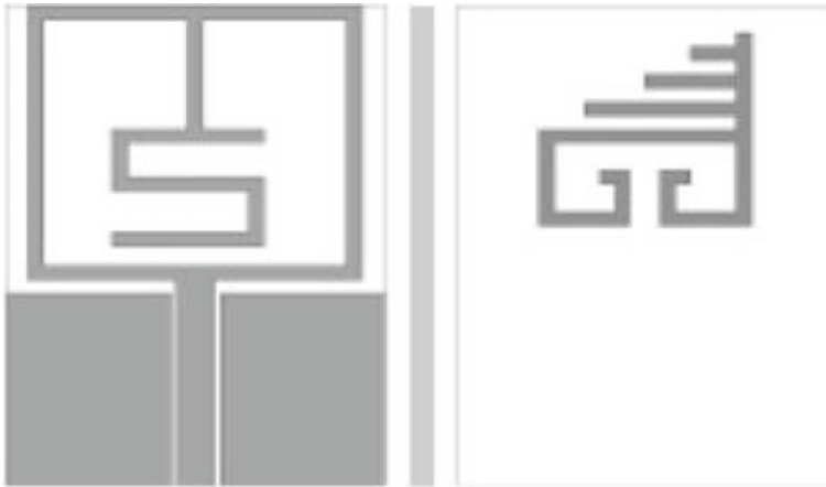
Fig. 8 Coplanar waveguide fed antenna
