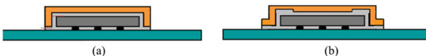
Fig. 15.13 (a) Potential failure modes for capped-die flip chip packages; (b) A capped-die flip chip package using an improved die cap design [66]
