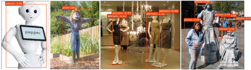
Fig. 2 Evaluation using model trained on PASCAL VOC 07+12 dataset: detecting robot, scarecrow, mannequins, and statues as person
