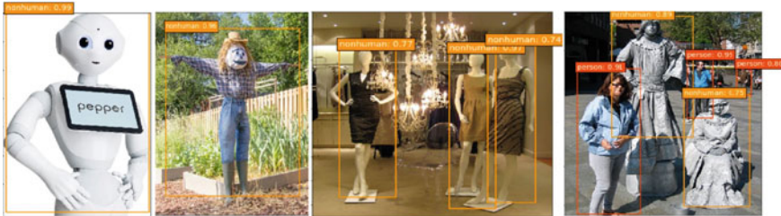
Fig. 3 Evaluation using model trained on PnPLO dataset: robot, scarecrow, mannequins, and statues are correctly detected as nonhumans
