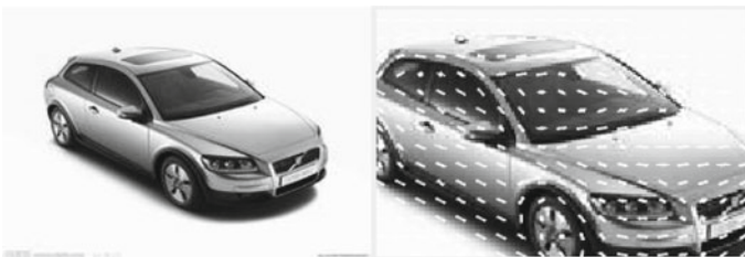
Fig. 3 Example of HOG features. The original picture is shown in left and the picture of HOG features is presented in right
