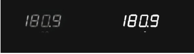
Fig. 3 Original subtraction image and the image after binarization using the Otsu method
