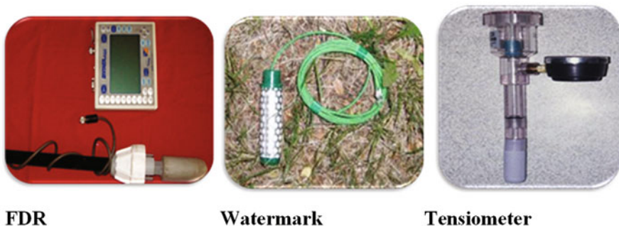
Fig. 15.18 Soil moisture sensors for irrigation scheduling
