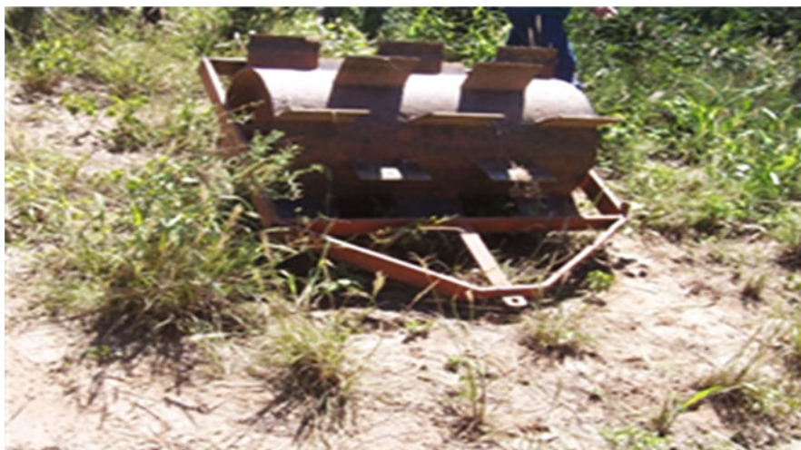
Fig. 14.4 Small roller for small surfaces can be pulled by tractor or animal traction
