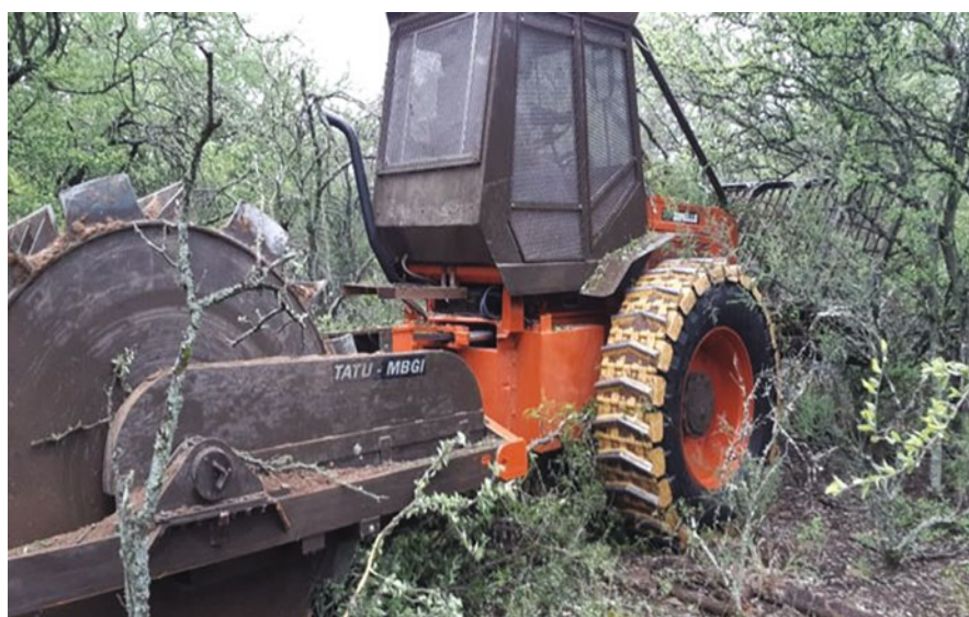
Fig. 14.6 Self-propelled roller recently developed by INTA
