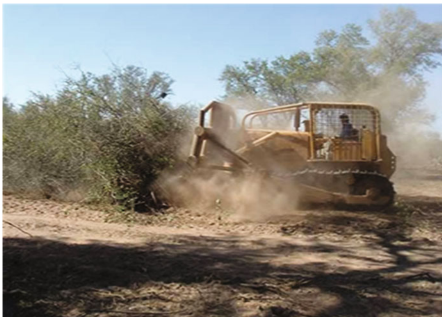
Fig. 14.5 Front roller, with hydraulic traction
