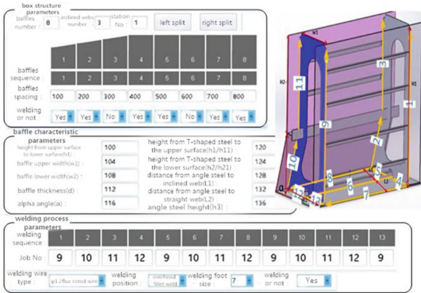
Fig. 5 Parametric programming interface for shaped box welding with robot
