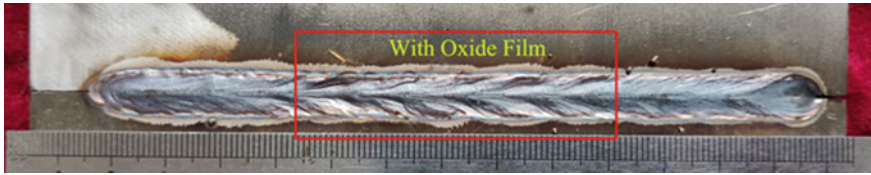
Fig. 7 Photograph of weld with oxide film
