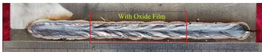
Fig. 7 Photograph of weld with oxide film
