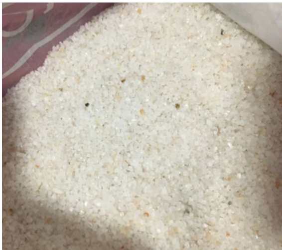
Photo 1 Fresh ennore sand
