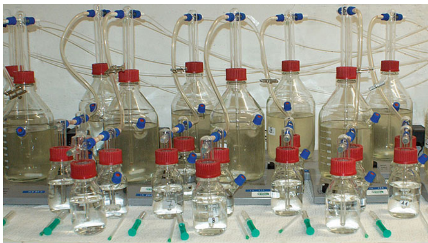
Fig. 4 Pictorial view of sturm test biodegradation being performed in laboratory
