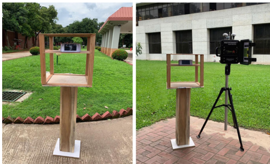
Fig. 2 AV pro with expedient frame during data collection and validation experiment with HIM 6000
