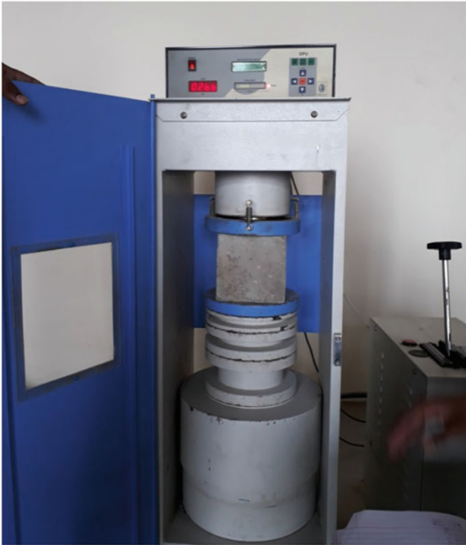
Fig. 4 The cube specimen placed in the testing machine
