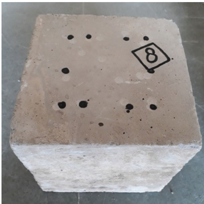
Fig. 3 Detailing of 10 points on each cube with a unique number
