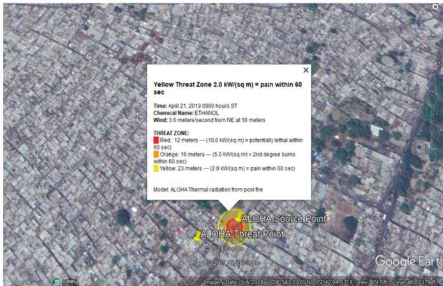
Fig. 2 Flammable, toxic area and thermal radiation due to dispersion of ethanol, wind speed 3.6 m/s
