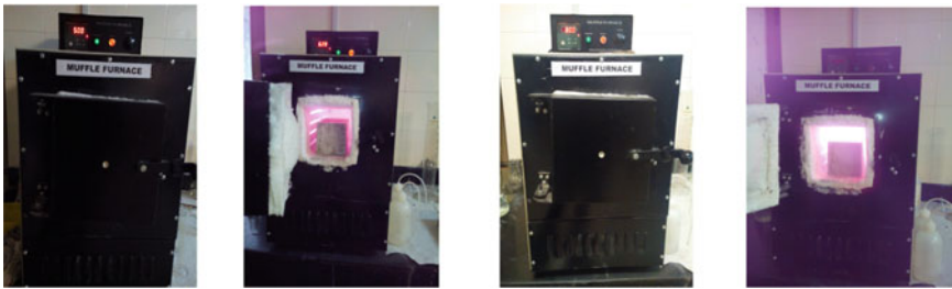
Fig. 2 Cubes incorporating alccofine at varying temperatures placed in muffle furnace
