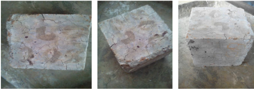
Fig. 4 Superficial cracks on cubes due to varying thermal gradient
