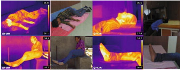
Illustrative set of visible and IR images of Positive class “presence of victim”
