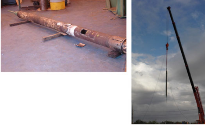
Fig. 19 Testing out torpedo-anchor with piezocone at Sarapui site (Porto et al. 2010)
