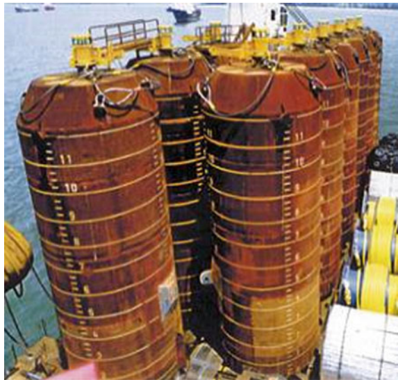
Fig. 4 Suction caissons: 5.5 m diameter by 13.5 long
