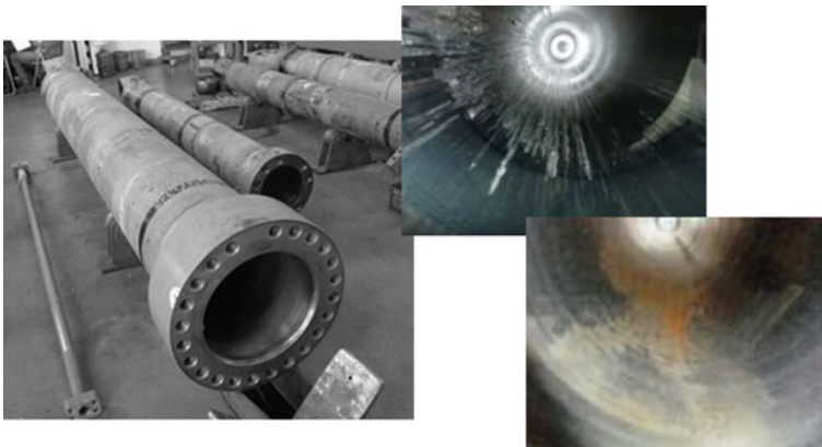
Fig. 36.4 Scratch and corrosion on hydraulic cylinder tube
