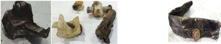
Fig. 8.5 Unliberated steel fasteners for same and different material combinations (Fe–Al, Fe–Plastic)
