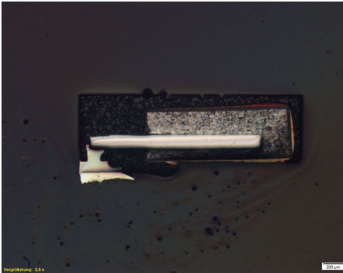
Fig. 26.10 Microscopy cross section of tantalum capacitor “Js” from Samsung Galaxy S7
