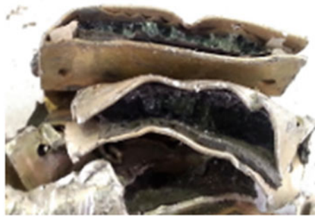
Fig. 8.3 Sandwich layer adhesion for different material types (Al-glass)
