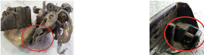
Fig. 8.4 Unliberated steel rivet from the car door mechanism and car door handle (aluminium)
