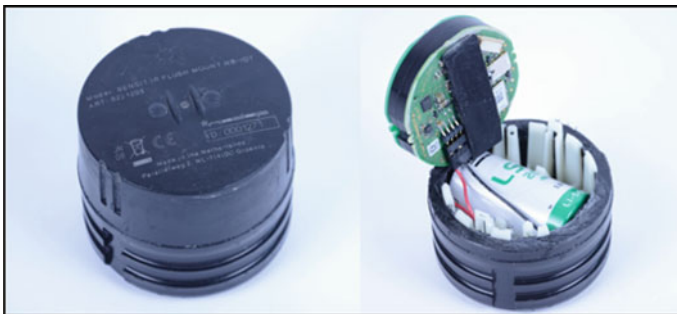
Fig. 26.1 Parking sensor closed (left) and open (right)
