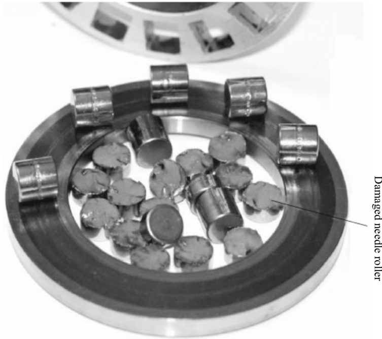
Fig. 9.6 Bearing damage picture
