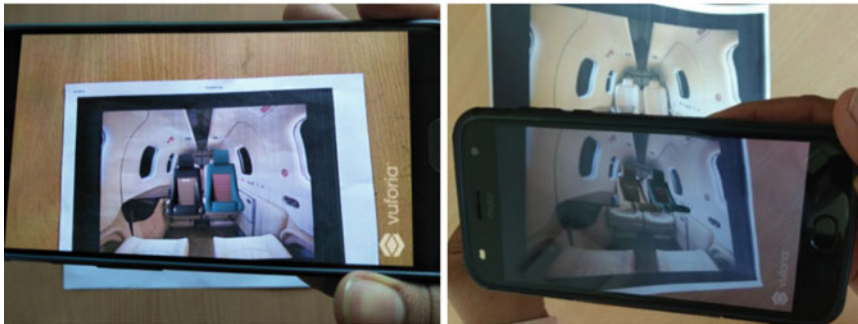
(b) Visualization of the augmented objects (e.g. seats on target object) by rotating the smartphone: Different views.
