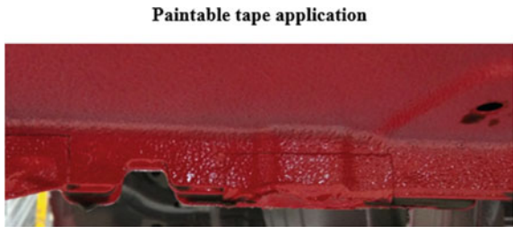
Fig. 5 Paint shop actions to stop or reduce body level air leakage
