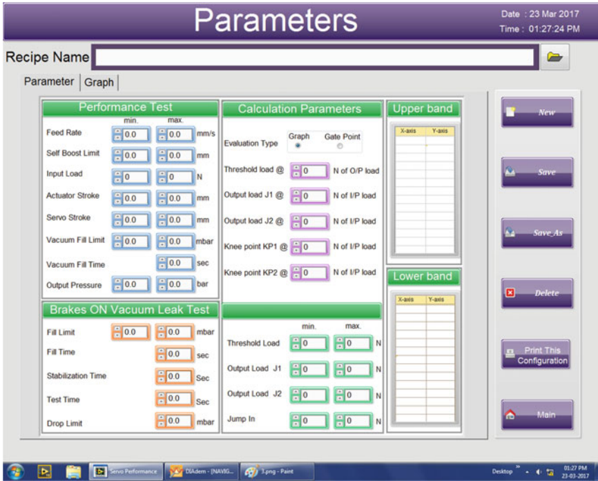
Fig. 2 Front panel of the vacuum booster—entering the parameters
