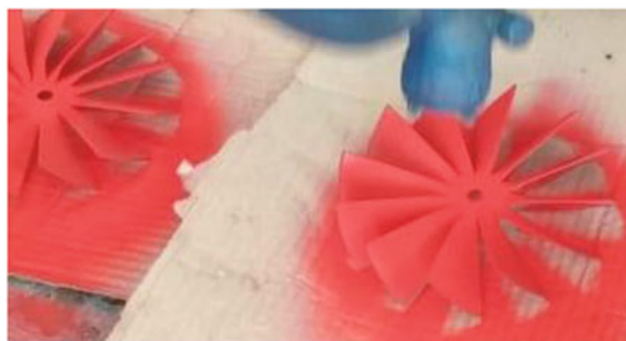
Fig. 6 Thermal paint sprayed blades
