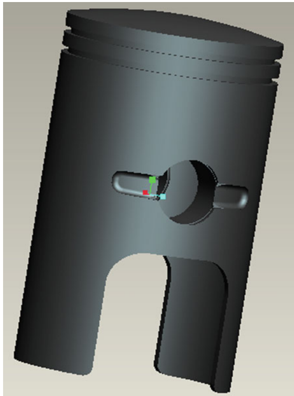
Fig. 3 Snapshot of 3D shape of the piston in Pro\Engineer
