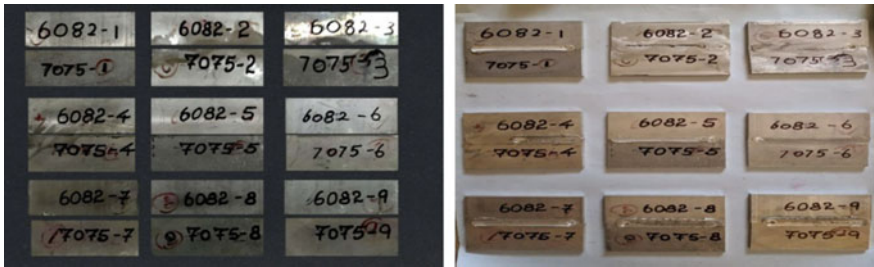
Fig. 2 Arrangement of before and after FSW joints
