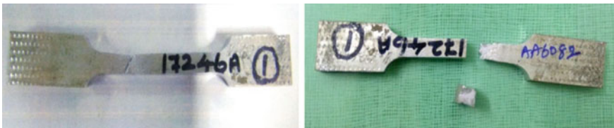
Fig. 3 Sample specimen diagram for before & after tensile test
