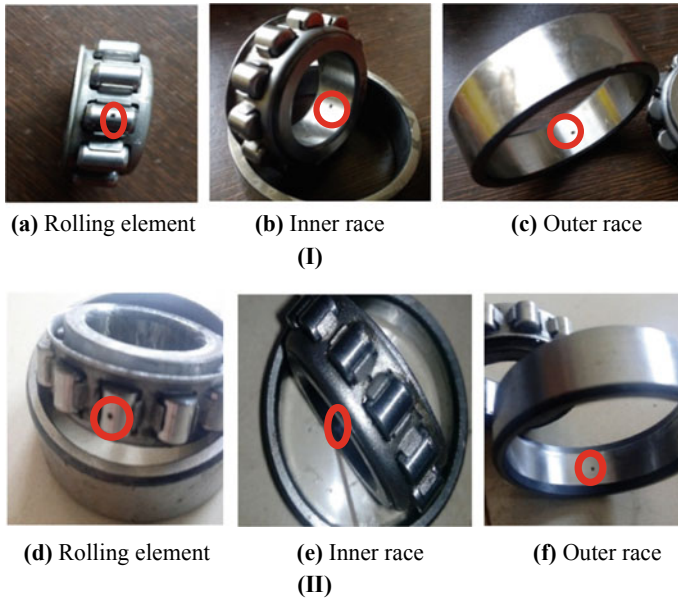
Fig. 4 Square defect on a rolling element, b inner race, c outer race. Circular defect on d rolling element, e inner race, f outer race
