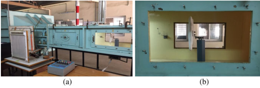
Fig. 7 Wind tunnel a equipment, b test division with model
