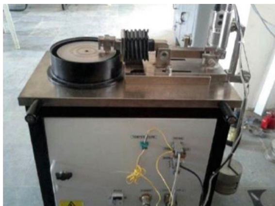
Fig. 9 TR10 LE model pin on disc wear testera
