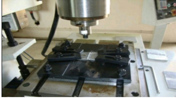
Fig. 1 Schematic diagram of FSW joint making process
