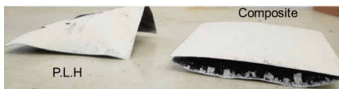
Fig. 5 Residue left after the cone calorimeter test, a Paint + Laminate + Honeycomb (P.L.H) and b Composite
