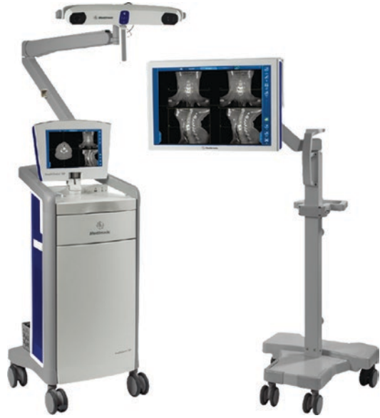
Fig. 1 Navigation system including work station, monitor, and infrared camera
