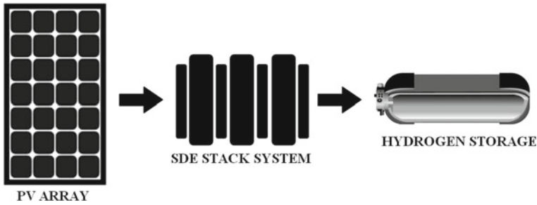
Fig. 61.1 Schematic diagram of the solar hydrogen production system
