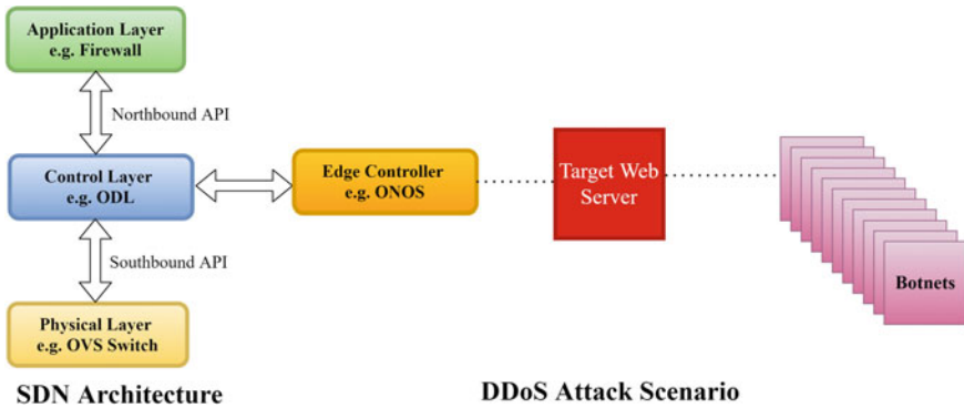
Fig. 2. Proposed framework to defend DDoS attack using SDN based architecture
