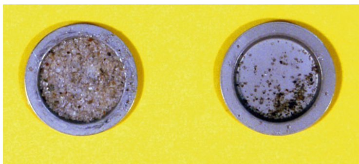
Fig. 4.2 Mineral fractions isolated from dried herbs in whole (left) and from spicy vegetal concentrate (right) on stainless steel TL measuring cups stabilized with silicon spray. Mean dimensions (diameter) of mineral grains ca. 140 nm (left) and ca. 80 nm (right) in diameter
