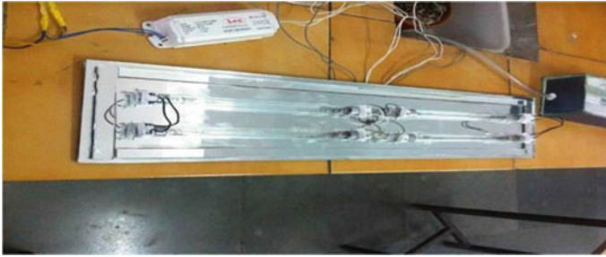
Fig. 5 Modified UV reactor with increasing intensity (Modified 3)
