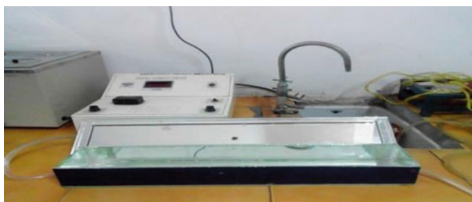
Fig. 4 Modified UV reactor with increasing length and decreasing height (Modified 2)
