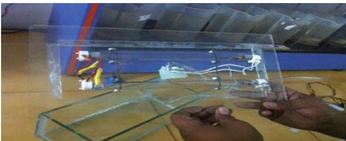
Fig. 2 Uncovered UV reactor
