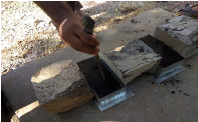
Fig. 3 Fabrication of paver blocks
