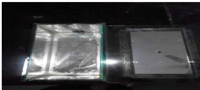
Fig. 3 Modified UV reactor with reflective mirrors (Modified 1)
