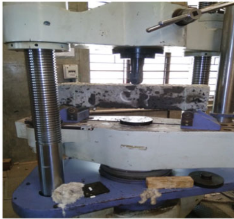
Fig. 3 Flexural testing using UTM
