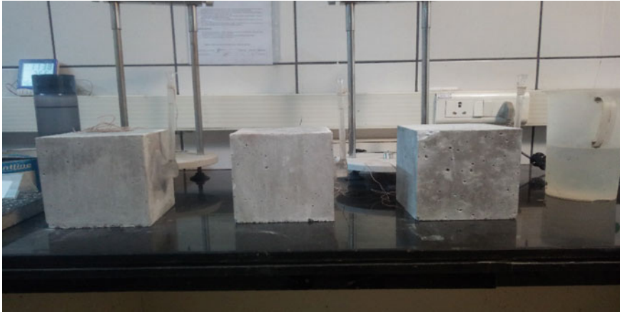
Fig. 6 Experimental setup of water absorption under low pressure
