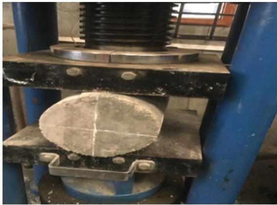
Fig. 4 Split cylinder tensile strength test
