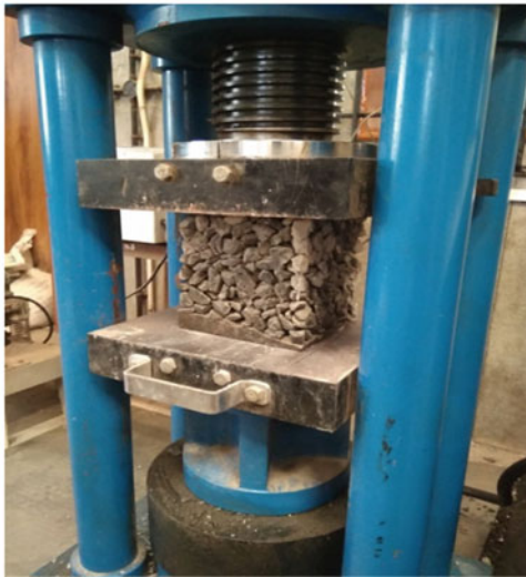
Fig. 2 Compressive testing using CTM
