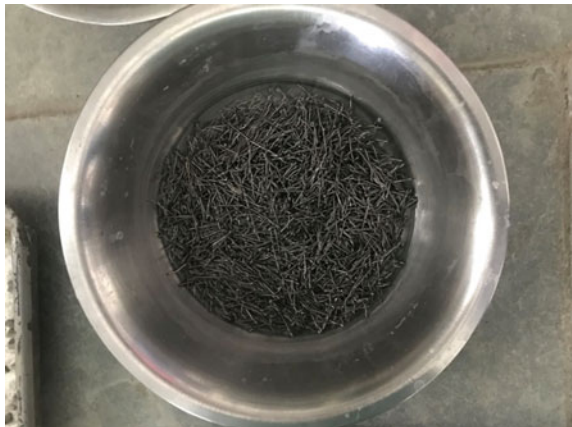
Fig. 1 Steel fibers immersed in NaOH solution
