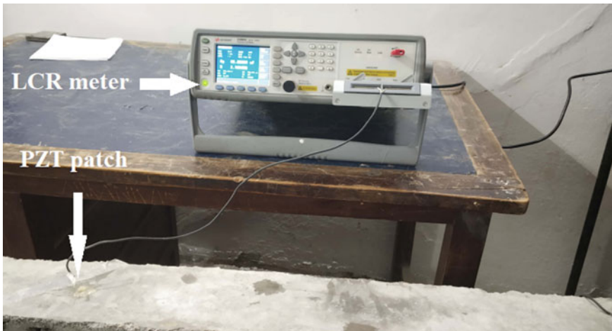
Fig. 3 LCR meter and PZT patch
