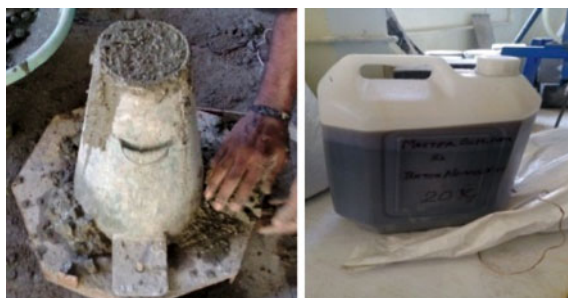
Plate 2 Slump test and glenium
