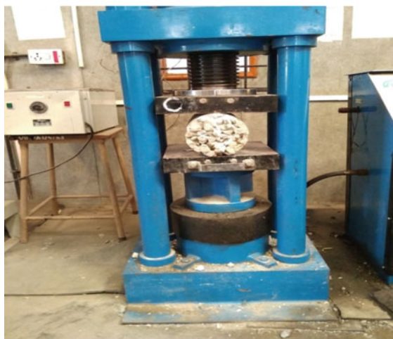
Fig. 4 Split tensile using CTM
