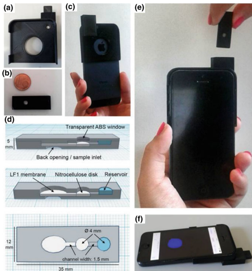
Fig. 7.1 a Picture of the accessory, b picture of the minicartridge, and c picture of the accessory snapped into the smartphone. d Schematic cutaway drawings of the minicartridge showing the integration of the various components. The transparent ABS optical window ( 200\ \mu\text{m} ) of 4 mm diameter allows imaging of biochemiluminescent reaction. e Introduction of the minicartridge into the accessory and f picture of a representative CL acquisition with the smartphone (Roda et al. 2014)
