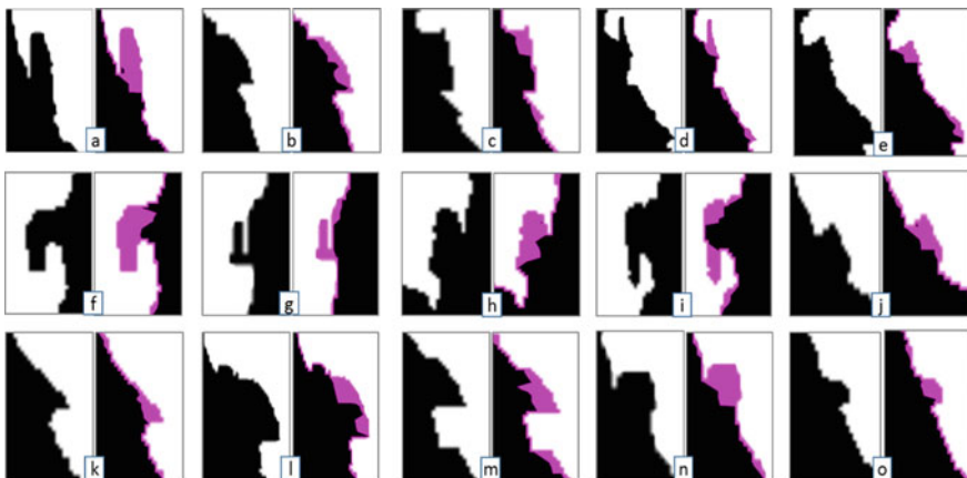
Fig. 8 Corrected binary mask images using the proposed algorithm (white regions show the actual segmentation having ridges and pits while the pink region shows the corrected binary mask)
