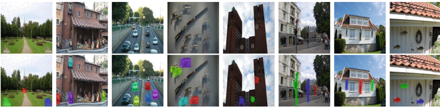
Fig. 7. First row corresponds to original images and second row is their corresponding localized region of original and forged images. These images are from MICC-F8 dataset.
