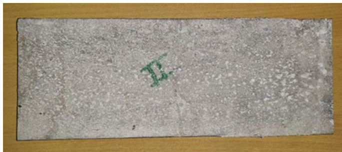
Fig. 7 Fabricated and corrosion tested sample 2
