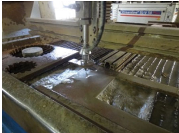
Fig. 1 Cutting zone of AWJ process
