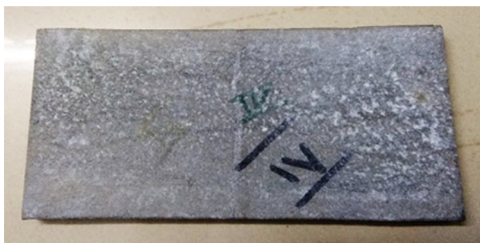
Fig. 9 Fabricated and corrosion tested sample 4
