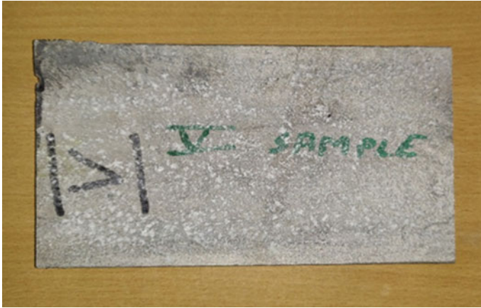
Fig. 10 Fabricated and corrosion tested sample 5
