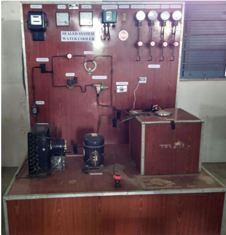
Fig. 1 Experimental setup of vapor-compression refrigeration system
