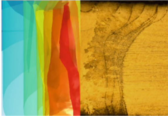
Fig. 5 Comparison of numerically simulated keyhole with 316L stainless steel joint
