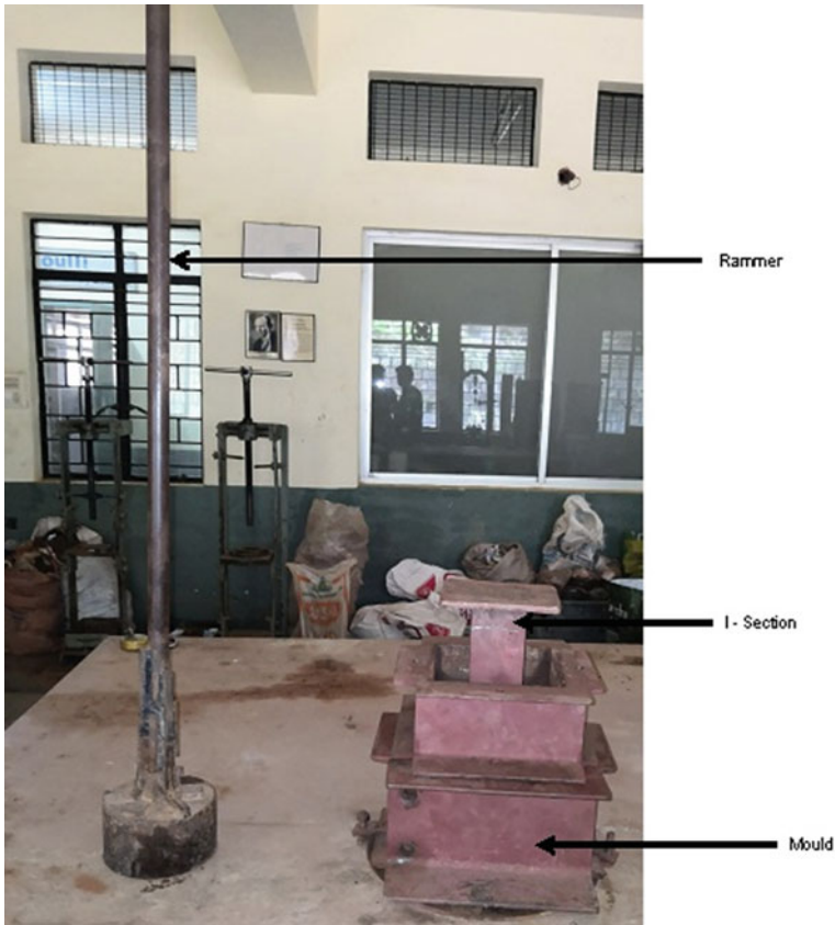
Fig. 4 Rammer, mould, collar and I-section used for compaction
