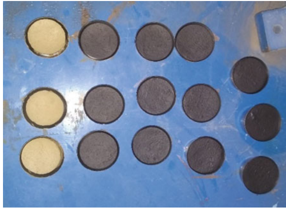
Fig. 7 Shrinkage limit test specimens
