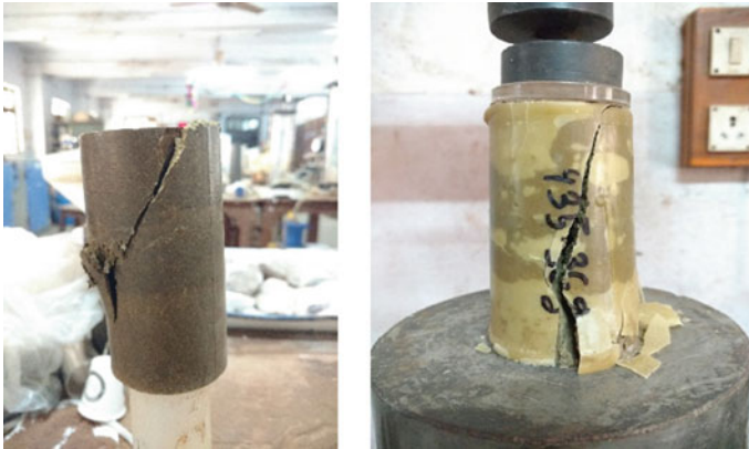
Fig. 10 Failure pattern of immediate and 28 days cured samples
