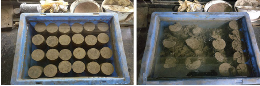
Fig. 11 Wetting cycle of treated (mix 12) versus untreated Soil
