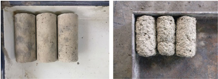
Fig. 12 Samples after 1st and 6th cycle, respectively
