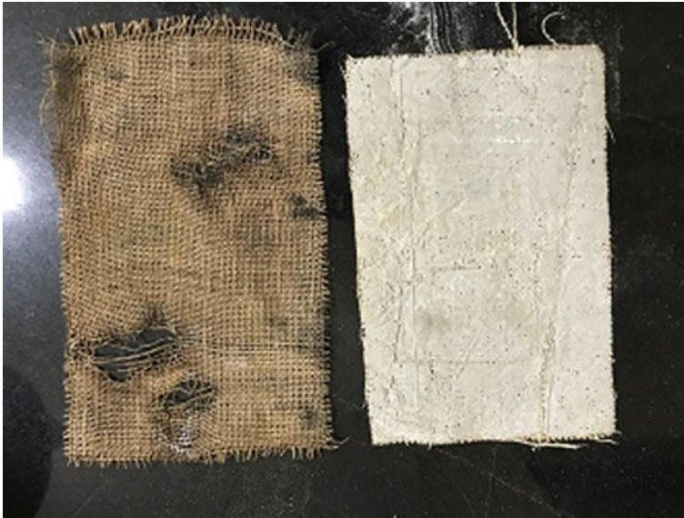
Fig. 5 Degradation of untreated jute geotextile (left) when compared to 0.35 w/s AAB treated jute (right) after exposure for 1 month in soil burial test
