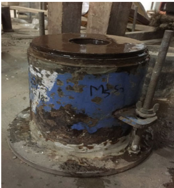
Fig. 7 Pasted CBR mould
