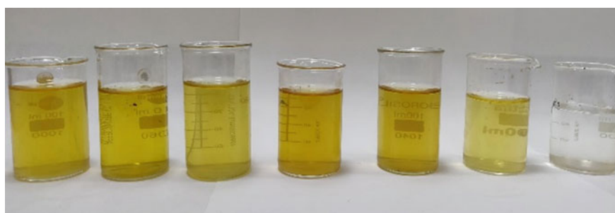
Fig. 3 Color of leachate released by SLM (L to R: Delhi location 1, Delhi location 2, Delhi location 3, Hyderabad location 1, Hyderabad location 2, Kadapa, Delhi silt)
