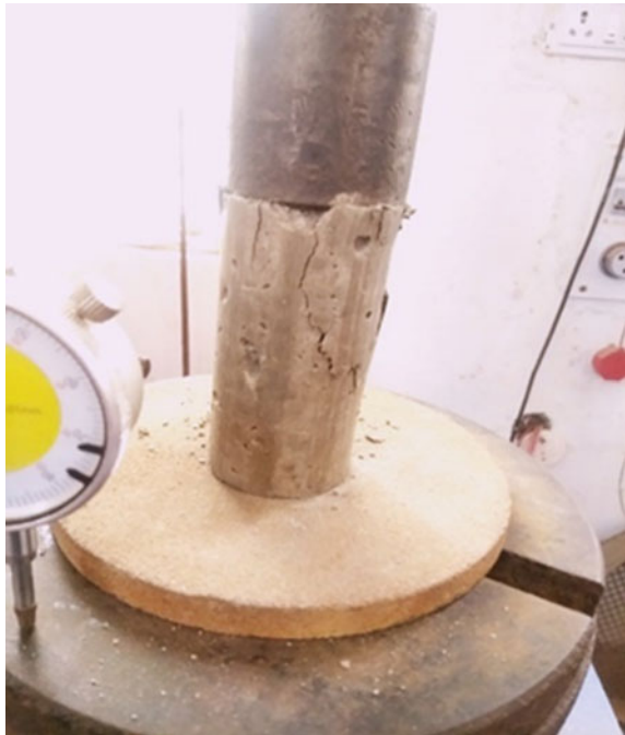
Fig. 3 UCC test result for I_c = 0.1 for different fibre content
