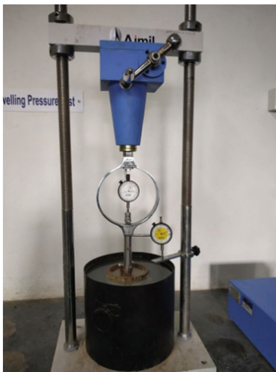
Fig. 5 Swell pressure test apparatus
