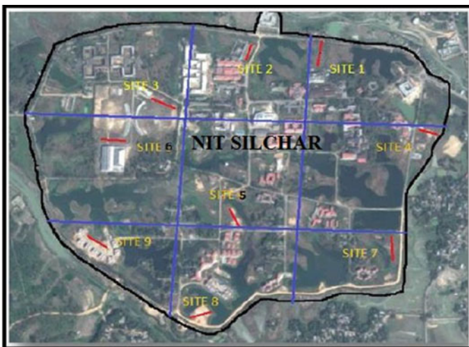
Fig. 2 Division of NIT Silchar into 9 grids and location of MASW test sites
