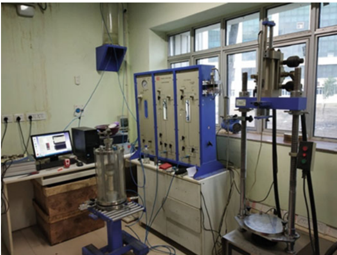
Fig. 2 Computer controlled cyclic triaxial test apparatus at IIT Patna used in this study
