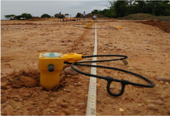
Fig. 3 4.5 Hz geophones being inserted into the ground surface for receiving seismic signals
