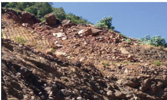
Fig. 12 Change in weathering condition of slope material along project roads in Ethiopia
