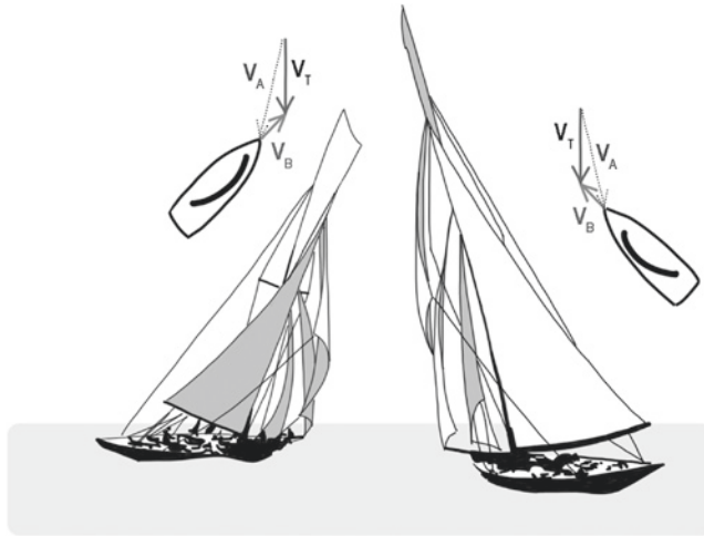
■ Fig. 4.11 Two sailing boats following a different course under the same wind conditions. The forward velocity reached by the craft ( V_B ) depends on the given true wind velocity ( V_T ) and the point of sail (boat course in relation to the wind). The apparent wind velocity ( V_A ) is the wind experienced by the boat in motion, and more specifically, it is the wind acting upon the leading edge of the most forward sail
