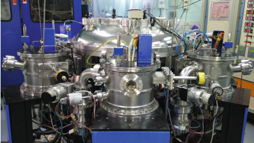
Fig. 8 HWCVD cluster tool used for the deposition of various doped and undoped silicon layers to avoid cross-contamination in the device structure. (Reproduced from Agarwal et al. [53])
