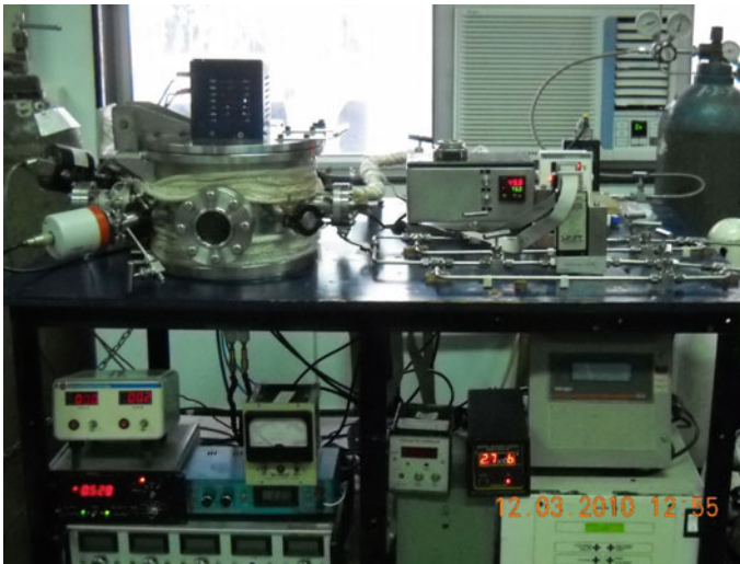
Fig. 2 The single-chamber HWCVD reactor with various control units
