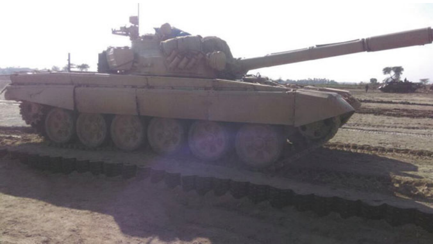
Fig. 12.16 Tank movements on geocell-reinforced track
