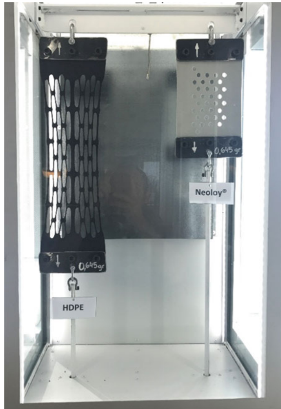
Fig. 3.1 SIM test showing creep of HDPE Geocell (left side) versus Neoloy Geocell (left side)
