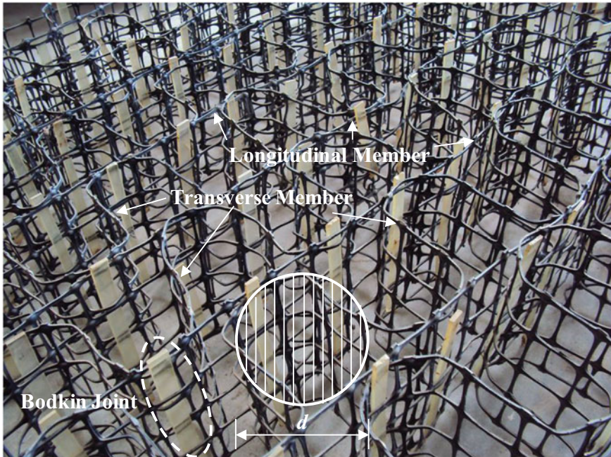
Fig. 6.4 Photograph of typical geocell-mattress in chevron pattern
