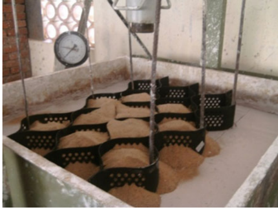
Fig. 18.3 Synthetic geocell as reinforcement
