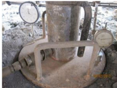
c Construction of geocell reinforced GSB layer and load test
