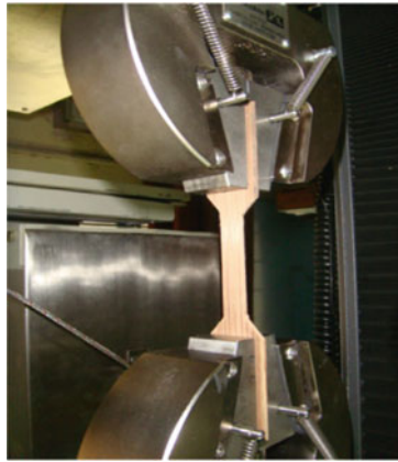
Fig. 17.5 Tensile test: a stress–strain behavior of different material (Sourced from Hegde and Sitharam 2015a with permission from ASCE); b bamboo sample during testing (sourced from Hegde and Sitharam 2015d)
