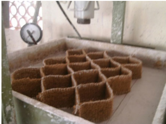
Fig. 18.4 Coir geocell similar to synthetic geocell as reinforcement
