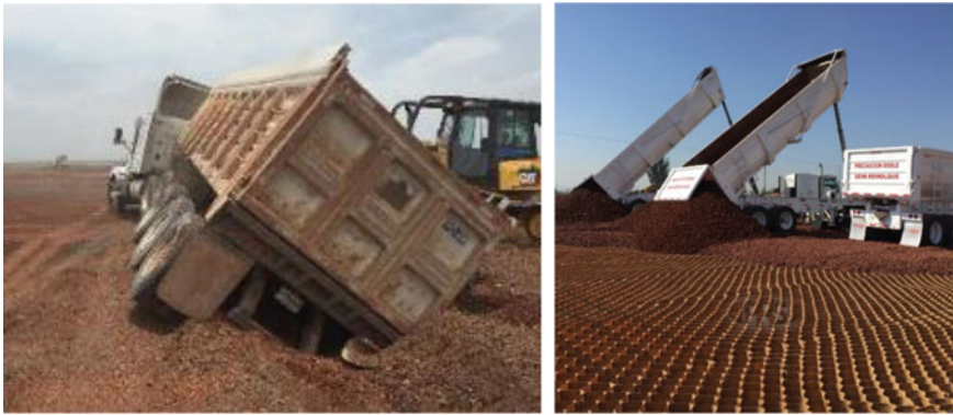
Fig. 15.3 Loaded truck in section reinforced with geogrids (left) versus section reinforced with Neoloy Geocell (right). Photo credit Innovater
