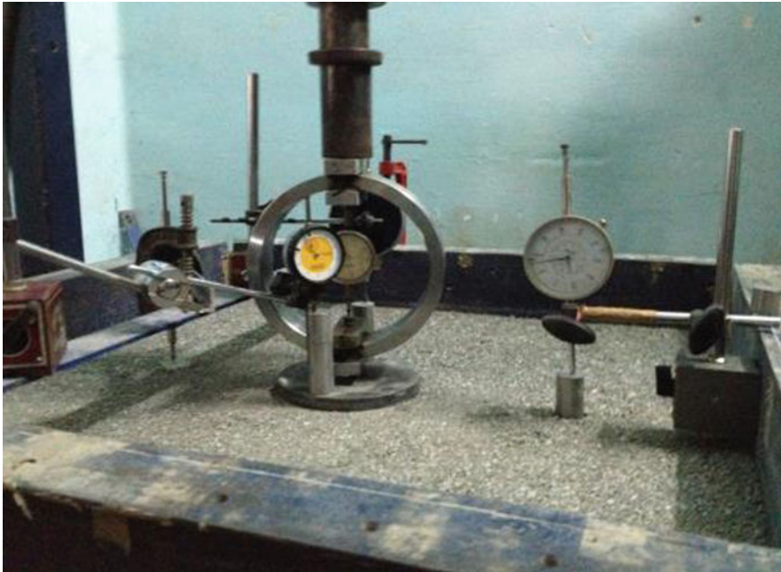
Fig. 10.5 Instrumented model section with construction waste as overlying fill
