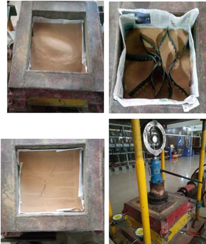
Fig. 12.6 Set-up for large-scale direct shear test used in present study
