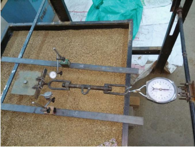
**Fig. 2** Actual setup of dial gauges; turn-buckle, spring balance and pile attached with pile cap
