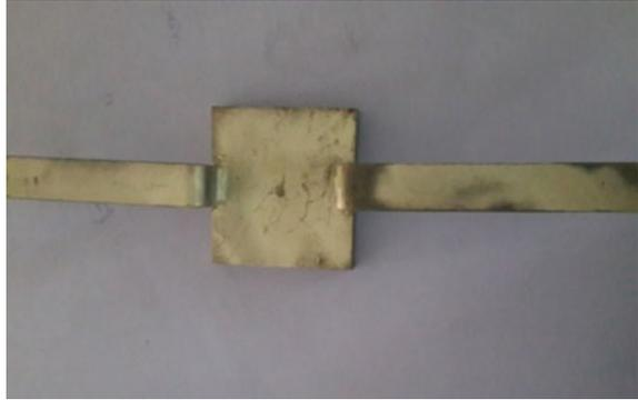
14.1 cm  $\times$  7.1 cm and 11.3 cm diameter, respectively. Every footing has a little groove at the center to facilitate the application of load. The base of the model footings was roughened by fixing a thin layer of sand to it with epoxy glue. The footings were provided with the two flanges on two sides of footings to measure the settlement of footing under the action of load with the help of dial gauges as shown in Fig. 2.
