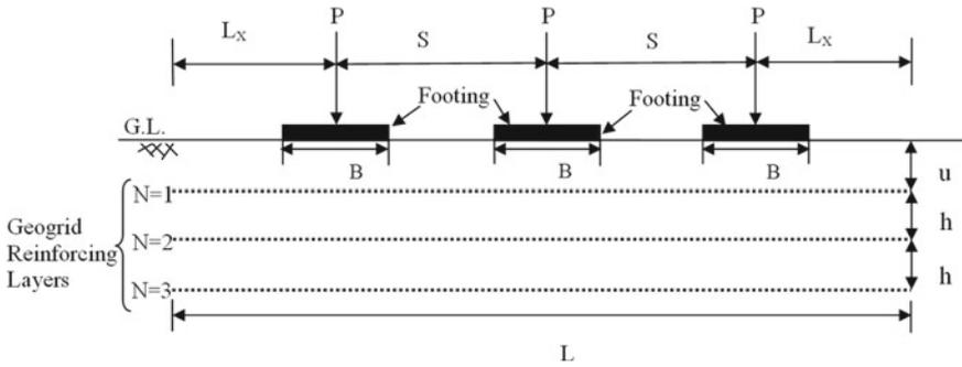
Fig. 1 Layout of geogrid reinforced sand bed
