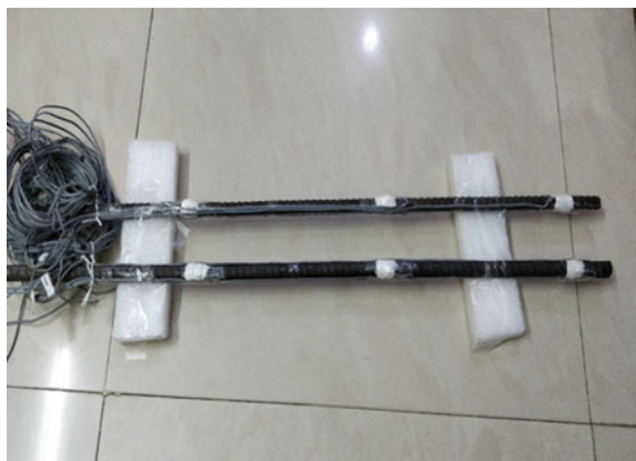
Fig. 1 Reinforcement after attaching strain gauges
