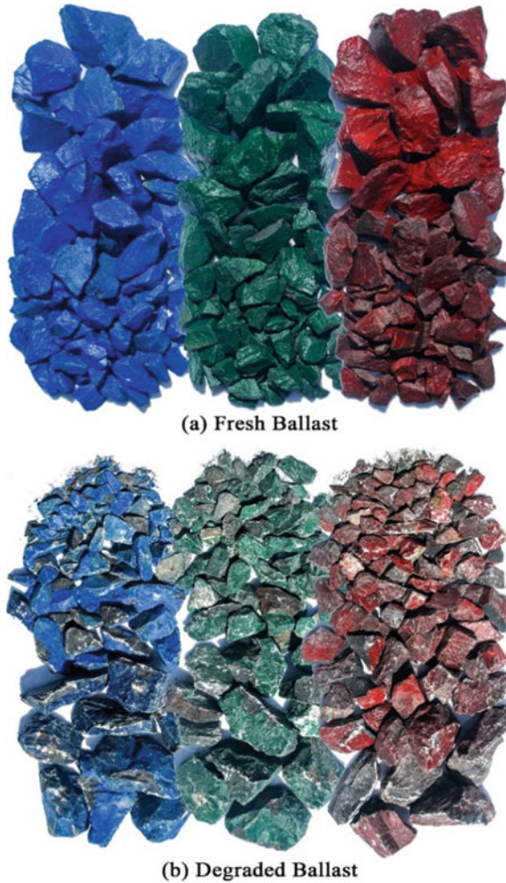
Fig. 9 a Fresh ballast before the test and b Degraded ballast after the test (modified from Navaratnarajah (2017))
