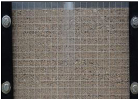
Fig. 3 Grid marked perspex sheet with sand infill and pile in background
