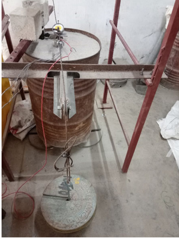
Fig. 4 Test setup for lateral load test
