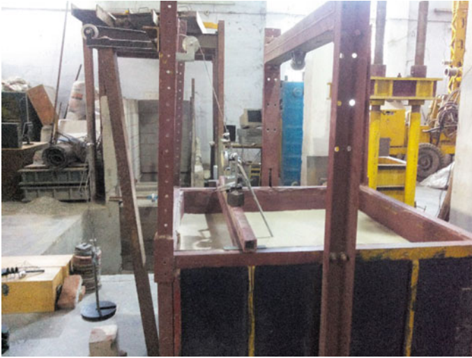
Fig. 2 Image of the setup after the application of the initial load to the inclined plate anchor in the sand box
