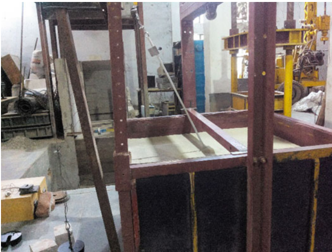
Fig. 3 Image of the setup after the application of pullout load at failure to the inclined plate anchor in the sand box
