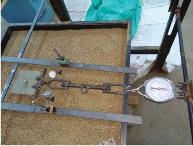
Fig. 2 Actual setup of dial gauges; turn-buckle, spring balance and pile attached with pile cap
