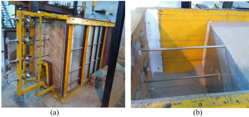
Fig. 2 Model test tank: a Proving ring arrangement, b Inside view of tank with titanium pipes
