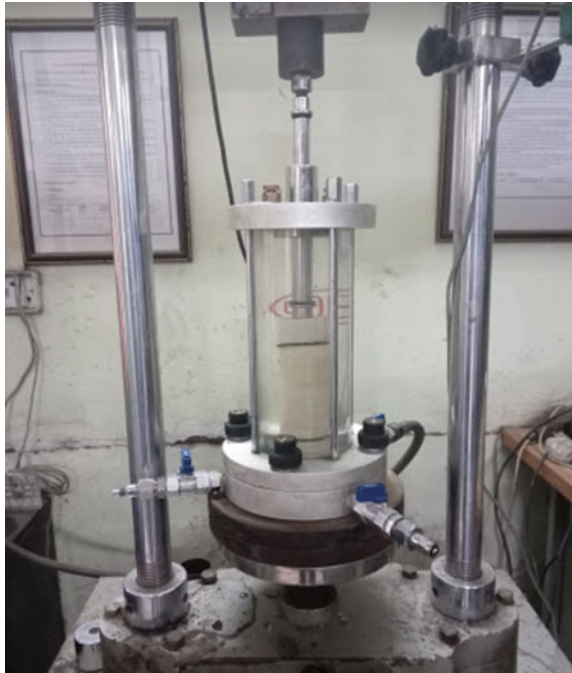
Fig. 5 Sample in a triaxial setup
